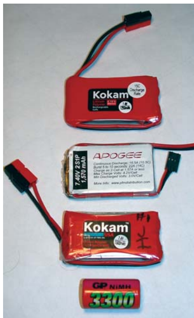
Three similar size and weight 2-cell Li-Poly cells. Top to bottom; latest generation Kokam 1250mAh pack (15C discharge rate), Apogee 1570mAh (14C) and the older Kokam 1500mAh (8C). All three packs would generally be used on models up to about 12-15 amps, but the older Kokam 1500 (8C) pack would be much happier at 8 amps. The old Kokam cells had a much higher internal resistance and could not sustain the voltage and capacity at these currents. GP-3300 NiMH cell for size reference.
