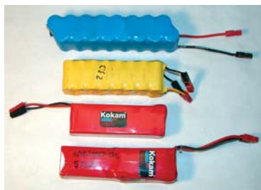
Top to bottom: The following packs were static and flight-tested in the 3D Gile-202 sport model; Sanyo 16-cell RC-2400 NiCd, Sanyo 16-cell 1950 NiMH, Kokam 5S 3200 Li-Poly and Kokam 5S2P 4000 Li-Poly. The data is presented in Tables 2 and 3.
