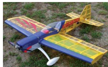
3D Giles-202 ( www.giantscaleplanes.com or www.chiefaircraft.com ) sport aerobatic model was used to static test four different types of batteries and flight test three of those same batteries. The RCATS flight data telemetry system transmitted and stored the data for analysis on the author's laptop computer. The packs tested were a Sanyo 16-cell RC-2400 NiCd, a Sanyo 16-cell 1950 NiMH, a Kokam 5S2P 4000 Li-Poly and a Kokam 5S 3200 Li-Poly. The data is presented in Tables 2 and 3.
