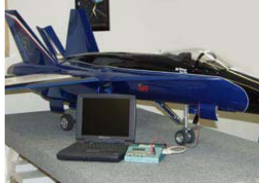
Batteries being cycled with an Orbit Charger and a R.S. 232 output to a laptop computer.
